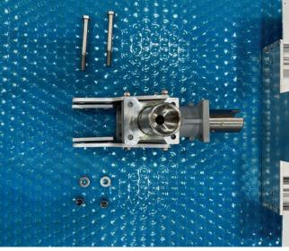
6. Mount the gearbox to the post and tighten all mounting bolts.
