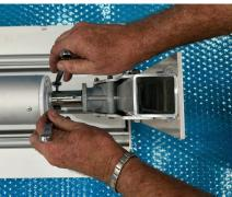
**10.** Lift the slave end and insert into the tube. Insert the mounting bolt then tighten.
