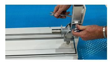
**7.** Prepare the tube for installation using the end slug with the hole to connect the gearbox using a 6mm bold and nyloc nut.
